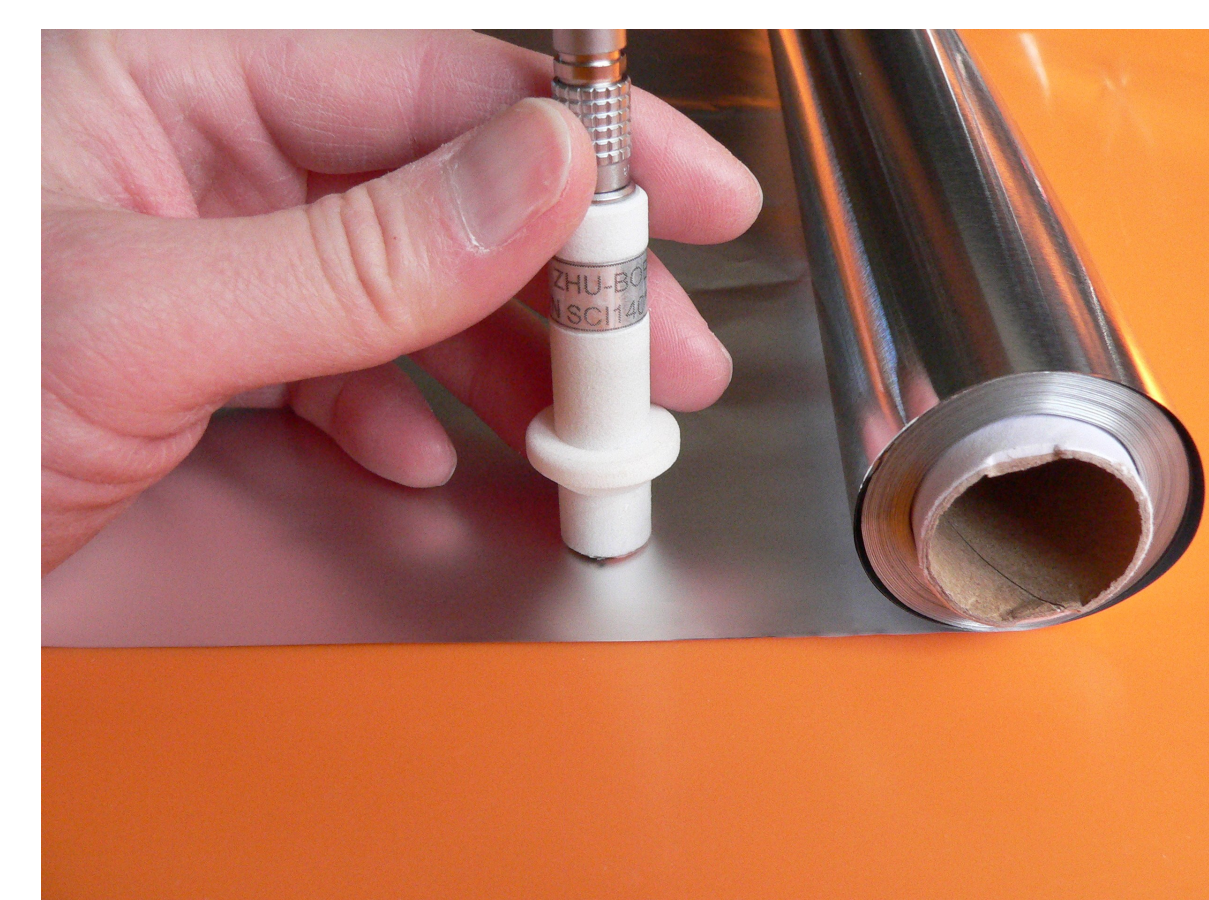
Checking electrical conductivity or thickness of thin metallic sheets or deposits
