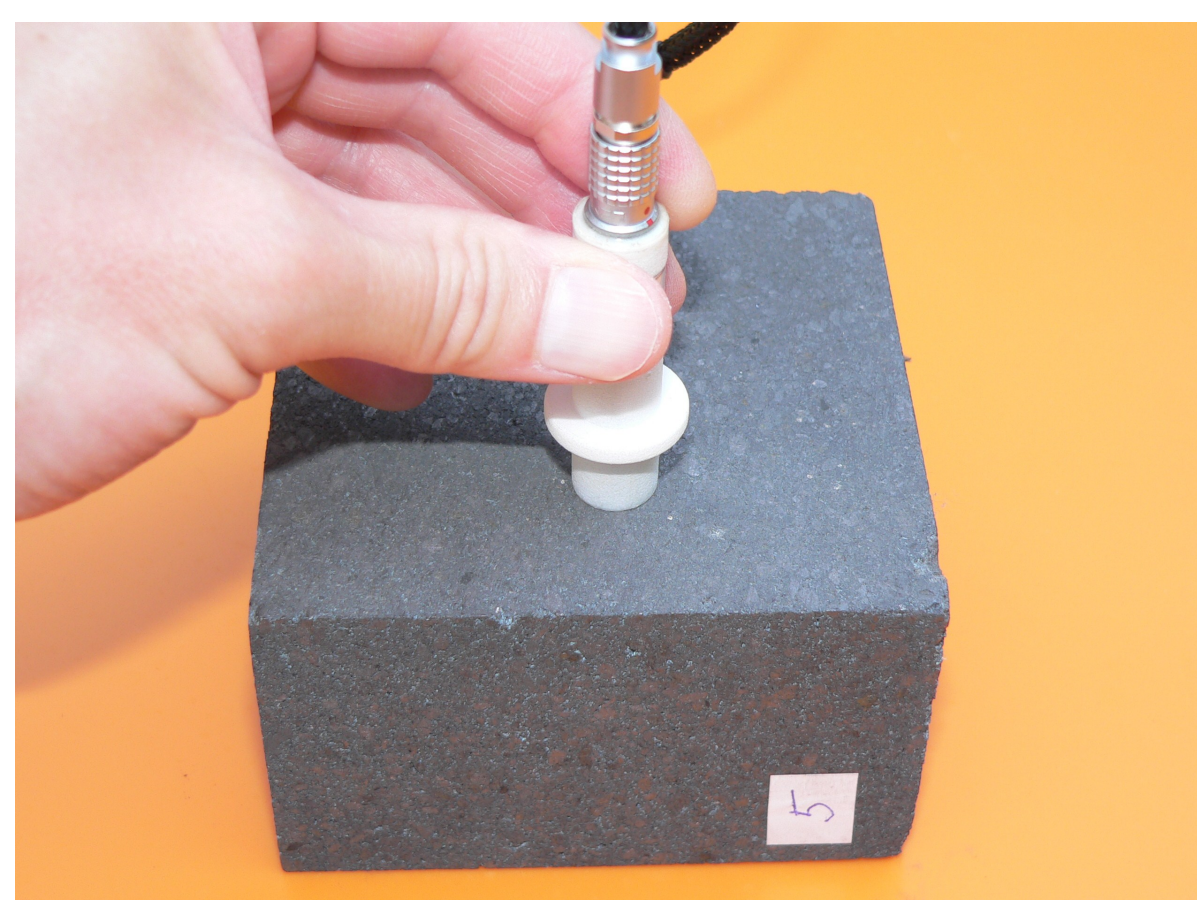
Checking electrical conductivity of graphite
