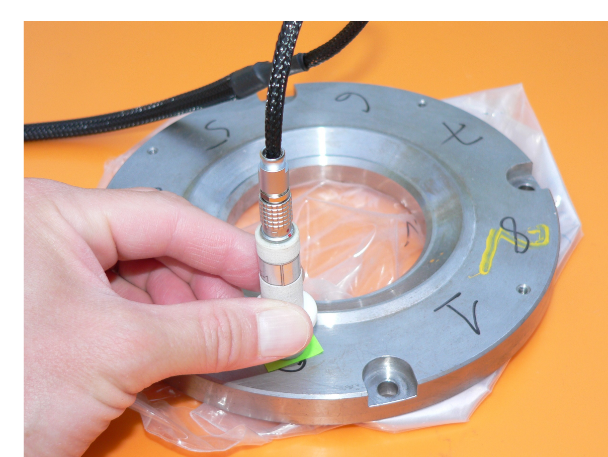
Checking electrical conductivity of machine parts made of steel
