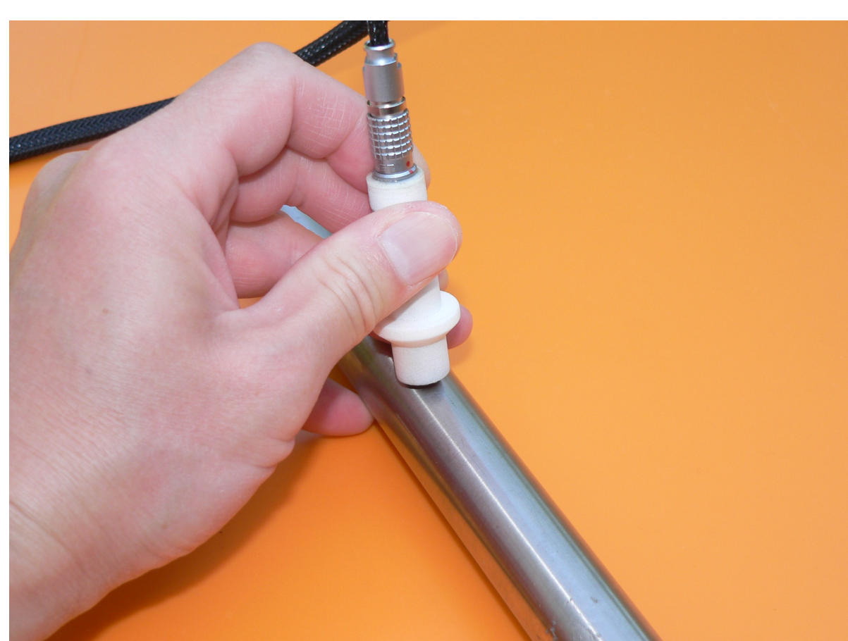
Checking wall thickness of steam generator tube
